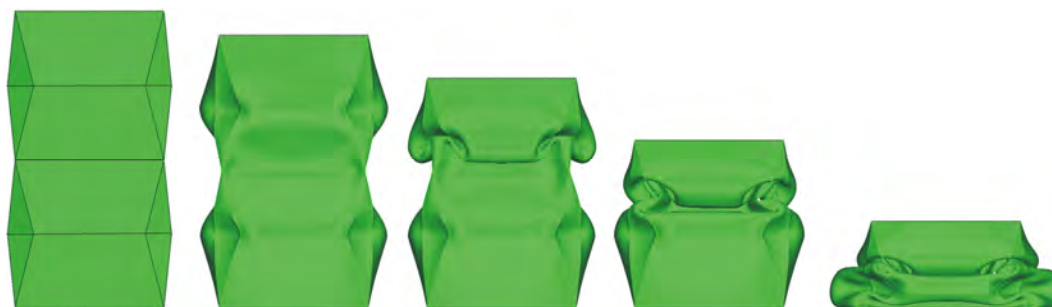
Fig. 4.14 Crushing process of A1_4.
