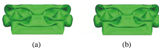
Fig. 4.29 Crushed configurations of A1_1 made of (a) high strength steel, and (b) aluminium alloy.
