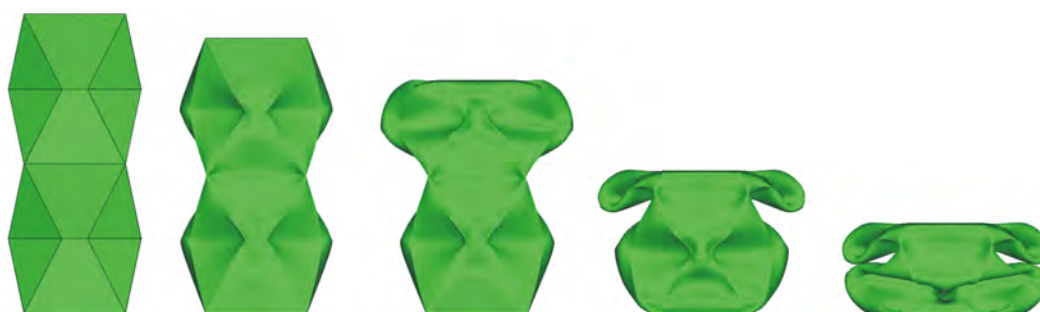
Fig. 4.18 Crushing process of B2.
