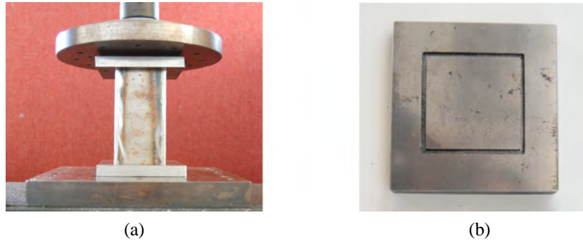
Fig. 3.4 (a) Pinned boundary conditions, and (b) a block with channels.
